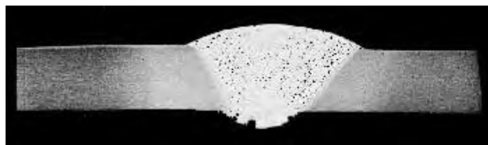
Figure 7: Porosity in aluminum alloy (Mathers, 2002)
