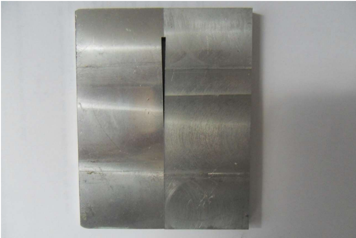
Figure 14: Cast alloy samples. Wrought alloy samples have the same design with different gap
