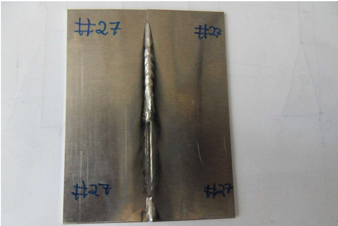
Figure 23: Bubbles with 1.75 m/min welding speed
