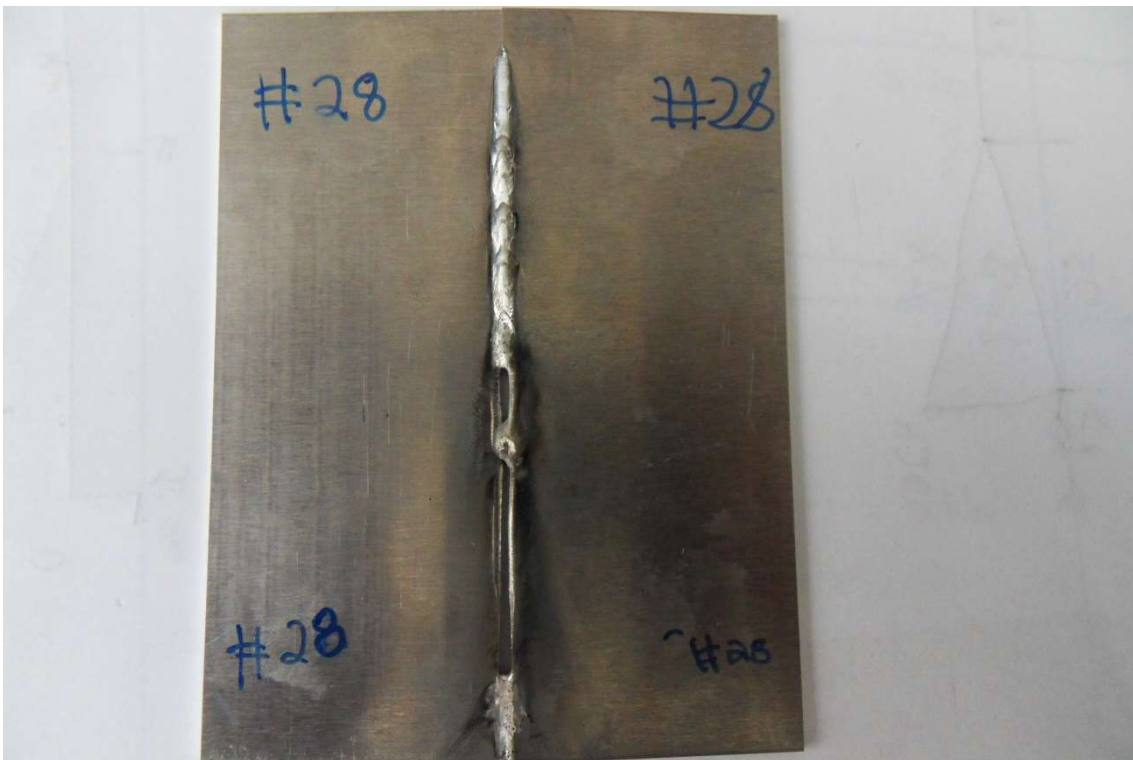
Figure 23: Bubbles with 1.75 m/min welding speed
