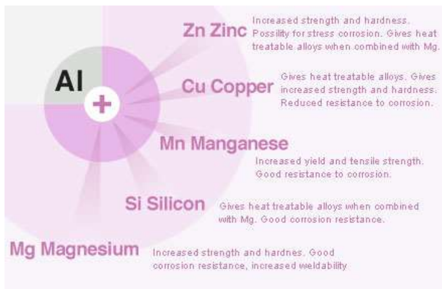
Figure 4: Alloying element influence in aluminum. Source: Aluminiumdesign.net
