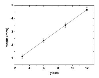
Fig. 2. Temporal evolution of the average depth of the wells. The symbols represent the average (squared) calculated for each of the inspections. The continuous curve is a linear fit whose Pearson's correlation coefficient is R = 0.999.
