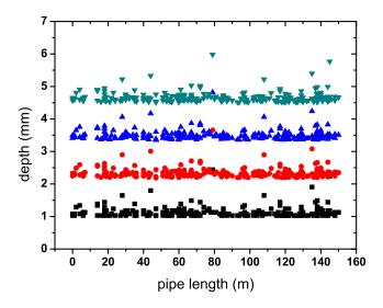
Fig. 1. (Color online) Distribution of depths of corrosion points along a 150 m section of a water service line. Each level observed in the graph corresponds to an inspection by MFL PIG. The four inspections were conducted over 12 years.
